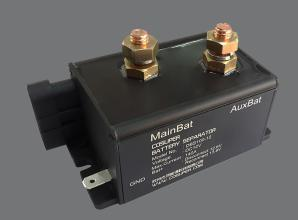
COSUPER battery isolator allows dual battery to be charged from single power supply such as alternator, battery charger or solar charger. Because of the unique ability of passing current in one direction, the first battery bank can be discharged without draining from the second battery bank.
